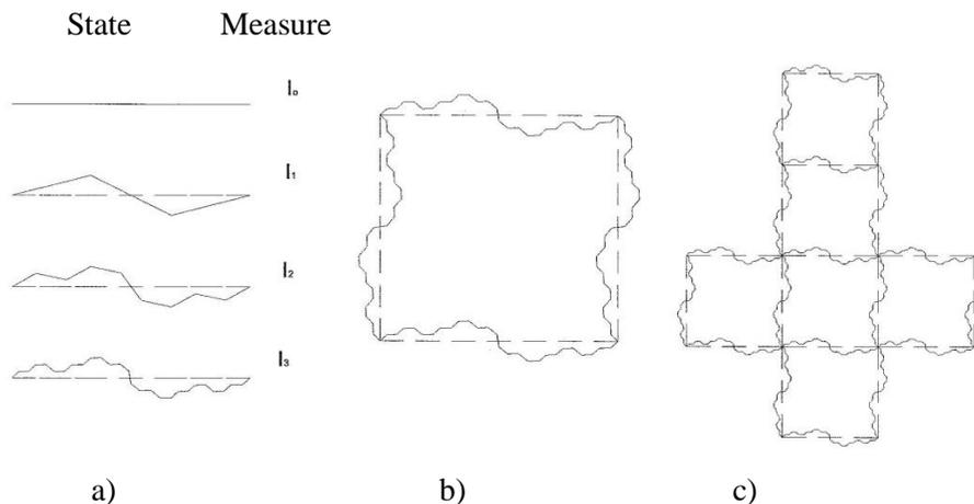
Figure 1. a) Construction of the fractal curve  $I$ . In every state  $I_k$  generator  $I_1$  is applied on every segment of the curve. b) Fractal curve  $I$  on the plane, and c) cubic form of fractal.
